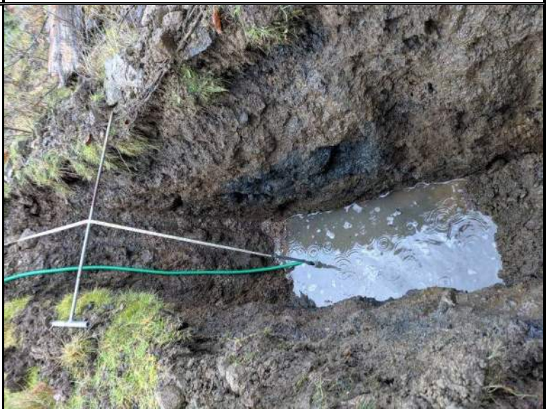
Infiltration test setup at test-pit P-1
